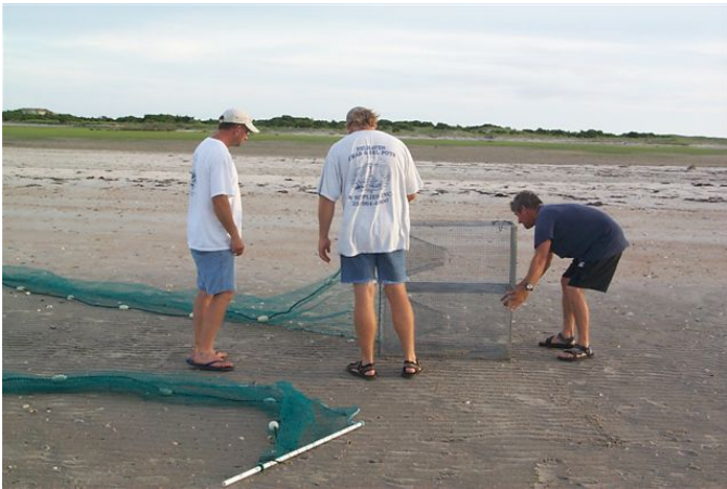
Experimental shrimp pot with leads attached.
