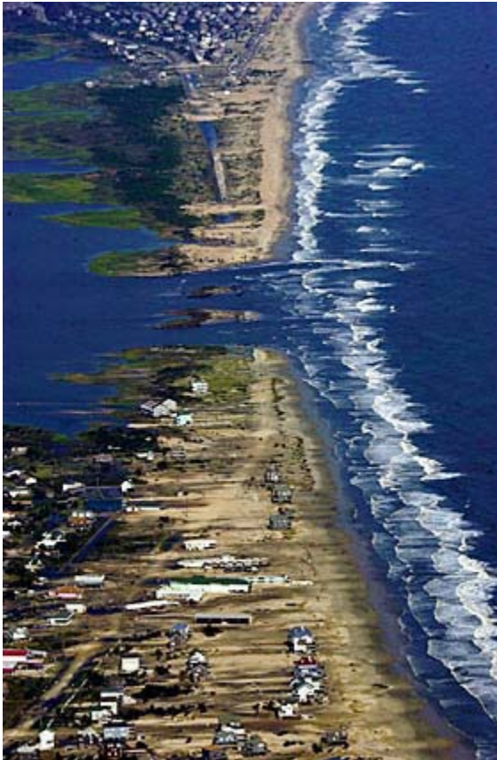
The new inlet formed by Hurricane Isabel between Hatteras Village and Frisco, NC. Note Highway 12 is completely gone. The inlet has since been filled in by the USACOE and Highway 12 has been restored.
